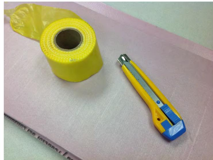
***Tools and Materials Needed When Working with Pink Board:*** Box cutter, various sizes of Pink Board, and a roll of Loc-Lift Rug Gripper Tape.
